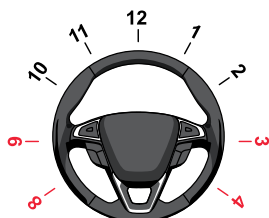
Hands holding the wheel at 9 and 3 o'clock are not as likely to be hit by the air bag.
